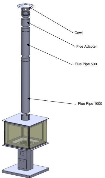
Fit Flue pipe sections and flue cowl as shown these are a push fit.
